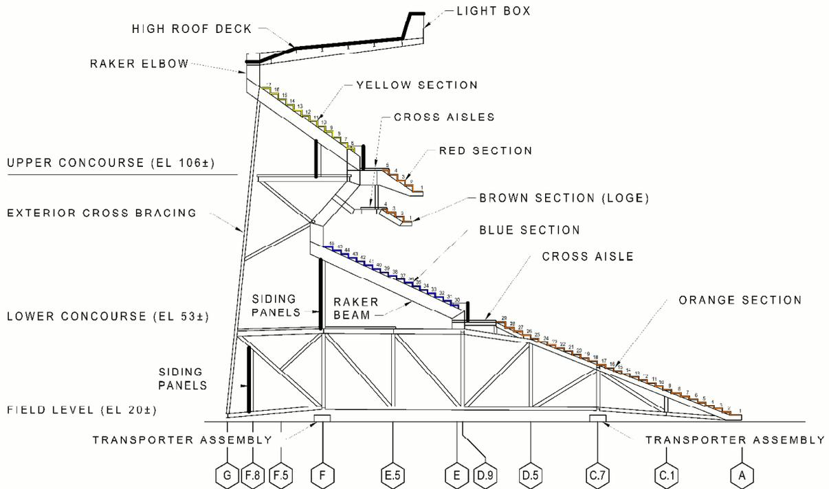
Figure 4. Schematic section through Aloha Stadium sideline seating stand structure.
