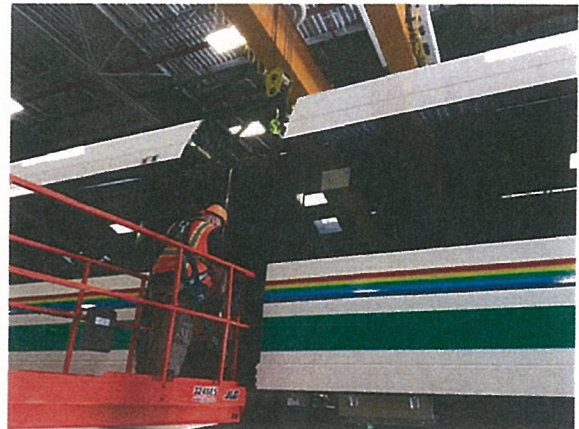
Installing Gangway Bellows
